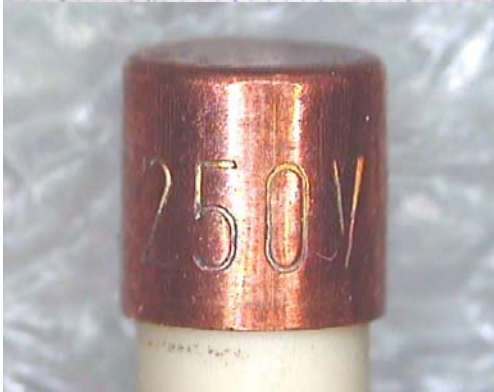
fig. 2: end cap with stamping of rated voltage and company logo (only on one end cap)
